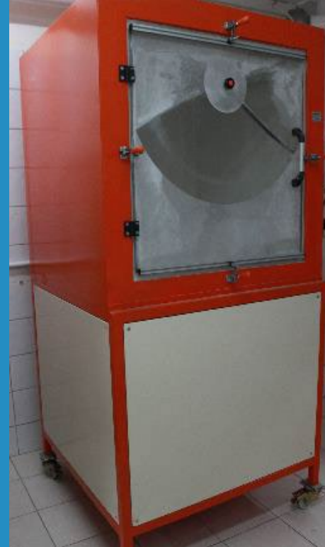
Dust Ingres Testing Cabin
